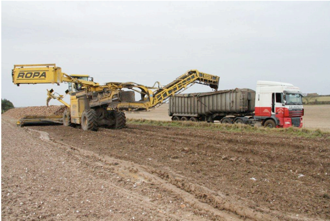
This sugar beet loader will load a lorry in 3 minutes
